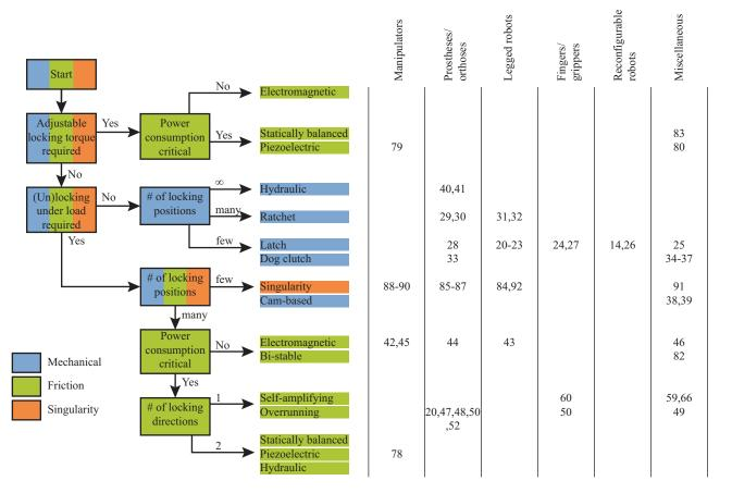
Fig. 5. Flow chart for selecting a locking mechanism. This chart will give the most specific locking mechanism. However, there might be application specific reasons to choose another mechanism. The references in which the mechanisms are currently used are listed on the right.
