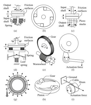
Fig. 3. This figure shows the types of friction based locking devices with: (a) a bi-stable brake, (b) an overrunning clutch, (c) a piezo actuated brake, (d) a statically balanced brake, (e) a wormwheel, (f) a self-engaging brake, (g) a thermic lock, (h) a self-engaging pinion-gear mechanism and (i) a capstan.
