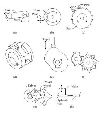
Fig. 2. This figure shows the types of mechanical locking devices with: (a) A latch with one locking position, (b), a latch with multiple locking positions, (c) a ratchet, (d) a dog clutch, (e) a cam-based locking device: cam follower, (f) a cam-based locking device: mutilated gears, (g) a cam-based locking device: geneva mechanism and (h) an hydraulic lock.
