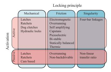
Fig. 1. Classification of the locking devices into three main categories: mechanical locking, friction-based locking and singularity locking. All three can be divided into actuated and passive devices.
