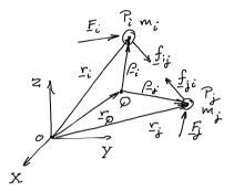
Figure 1.6: Definitions of the absolute and relative position of particles i and j, as well as of internal and external forces acting on the particles.
