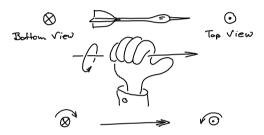
Figure 1.3: Notation for a vector that is perpendicular to the plane of drawing imagined as a dart (top); the right-hand rule to indicate positive direction of a rotation/moment about an axis (center and bottom).
