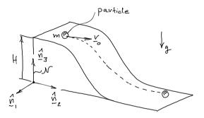
Figure 2.3: A particle sliding down a slide.
