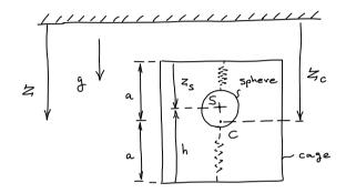
Figure 2.5: Simplified 1-D case of the accelerometer.
