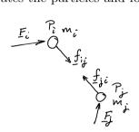
Figure 1.5: Two particles i and j with internal and external forces acting on them.
