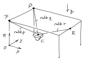
Figure 1.19: Camera suspension system
