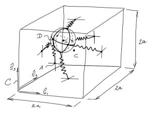
Figure 1.28: An accelerometer, consisting of a spherical mass suspended in a (transparent) cube by six springs.
