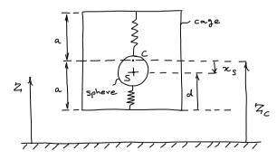
Figure 1.29: Kinematic diagram of simplified accelerometer in 1-D.
