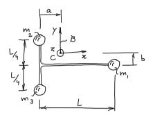
Figure 1.20: T-shaped rigid body consisting of three particles.
