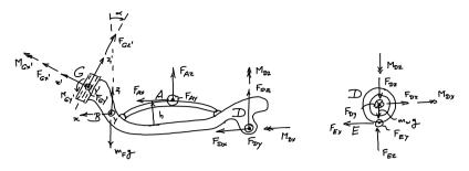
Figure G.5: FBDs of the scooter's footboard and rear wheel.
