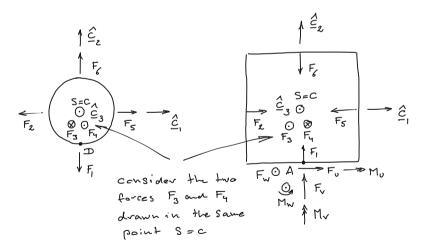
Figure G.4: Free-body diagrams for the accelerometer.
