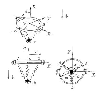
Figure 2.6: Catapult made with a ring, a cup to hold an object, and springs.
