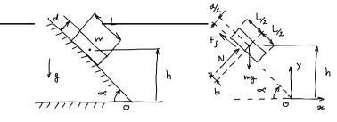
Figure 1.8: Sliding block and corresponding FBD.
