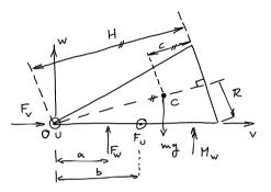
Figure 1.13: Exemplary FBD for the rolling cone.
