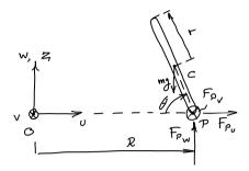
Figure G.1: Disk free-body diagram.
