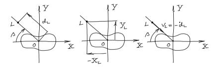
Figure 1.15: Describing kinematics of the lion. Left: Location in terms of distance and angle. Center: Cartesian coordinates. Right: Velocity
