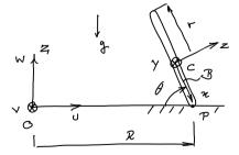
Figure 1.11: A disk rolling in a steady motion.
