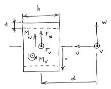
Figure 1.10: Free-body diagram of the ring.
