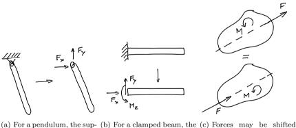
(a) For a pendulum, the support is replaced by forces transmitted by the hinge joint.
