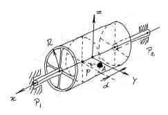
Figure 1.21: Unbalanced rotor.
