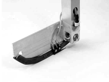
Figure 6.3: In practice, we obtained the best results with a foot radius of 25 cm, a foot length of 13 cm, and a forward displacement of 6 cm. The foot switch allows the controller to adapt to the actual step time by registering the exact instant of heel strike.
