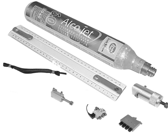
Figure 7.6: The pneumatic components and a 30 cm ruler to indicate their sizes. The components are clockwise arranged according to the \text{CO}_2 flow through the system; 5.8 Mpa \text{CO}_2 canister, the first stage pressure regulator to 1.2 Mpa, a block of four second stage regulators to 0.6 Mpa, one of four low-power SMC TM valves, one of four small SMC TM cylinders and one of four Shadow TM McKibben muscles.
