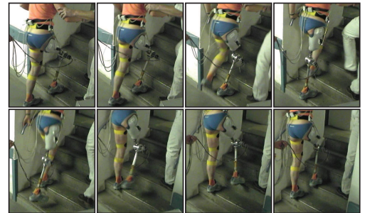
Fig. 5. Stair ascent with a CLME-controlled prosthetic knee joint. An assisting person (right) helps with balance. Time between adjacent frames: 40 ms.
