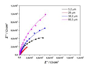
Nyquist plot (EIS) after potentiostatic polarization at  $0.4\ V_{Ag/AgCl}$  for 6 hours. The semi-circle size indicates the charge transfer resistance that decreases with PAGS refinement up to a critical value while further refinement leads to an increase
