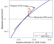
Fig 1. Extraction of the LPR value from the I-V curve.
