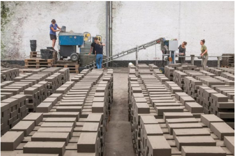
Photo from process of compressing earthblocks at the site. | Photo: © BC Architects.
