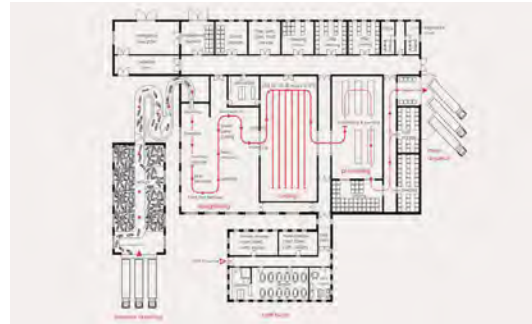
Schematic floor plan of industrialised slaughterhouse Source: Deutinger T. Handbook of Tyranny. Zwitserland: Lars Müller; 2018.
