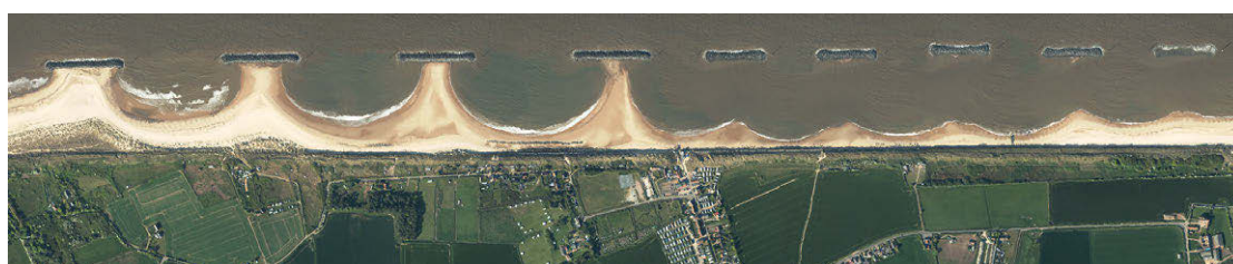
Figure 10.17: Series of emerged detached breakwaters in Sea Palling, England. Note the salients and tombolos. Vertical aerial photography obtained in May 2019. From UK Environmental Agency ('Credits' on page 579).
