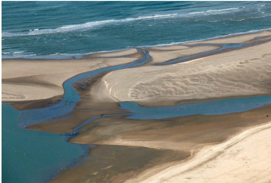
Figure 7.9: Ridge (intertidal bar) runnel (drainage channel) structure at low water at the northern flank of the Sand Engine on 16 February 2016. Photo by Jurriaan Brobbel, Rijkswaterstaat ( ‘Credits’ on page 579).
