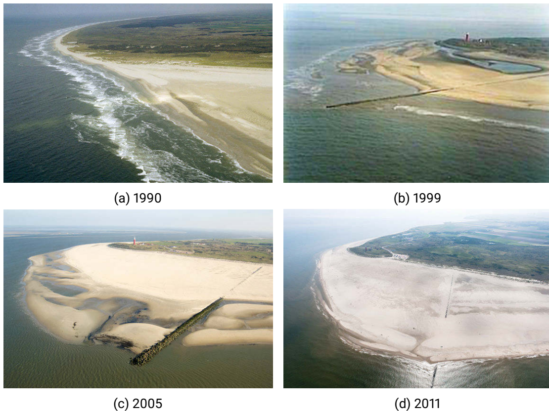
Figure 9.14: Observed morphological evolution around the Eierlandsedam, a long groyne at the north point of Texel built in 1995. Photos from Rijkswaterstaat (see 'Credits' on page 579).
