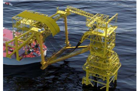
Figure 1. Soft Yoke Mooring System
