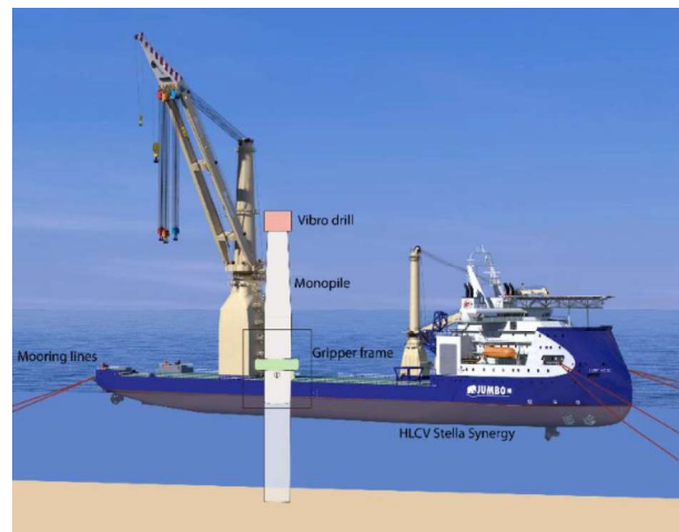
Figure 1.1 - Early Driving phase of a monopile installation
