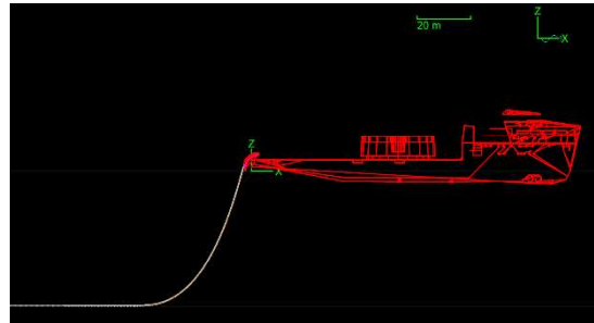
Figure 1: Static configuration of the base case model in Orcaflex.
