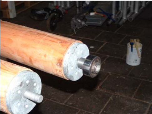
prestress auxiliary device
