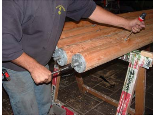
assembly of the connection
