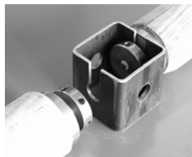
mounting of beams on chaining block
