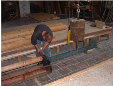
'workmanship' application of prestress in connections
