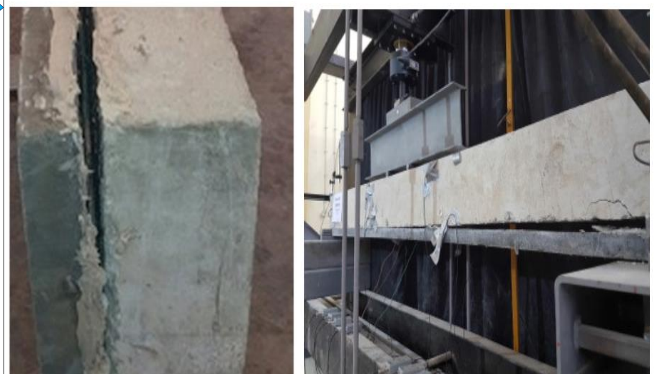
Interface formation and potential interfacial debonding
