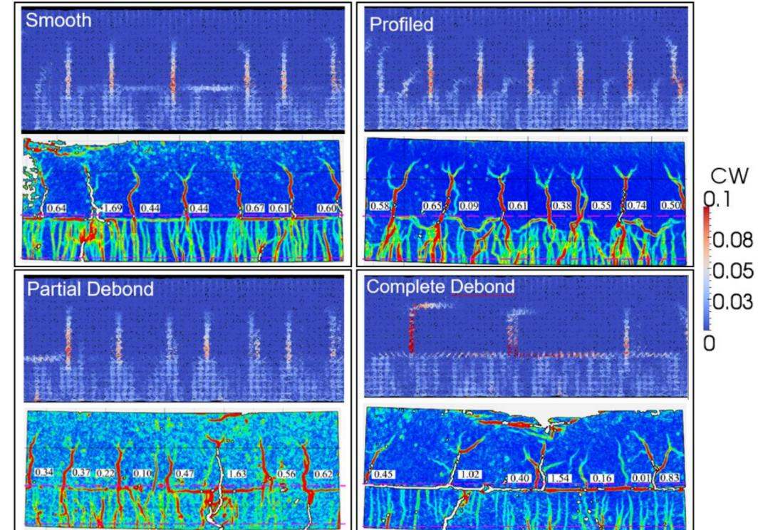
Hybrid beams with smooth and rough interface limit cracks below 0.3mm until yielding of reinforcement!!!
