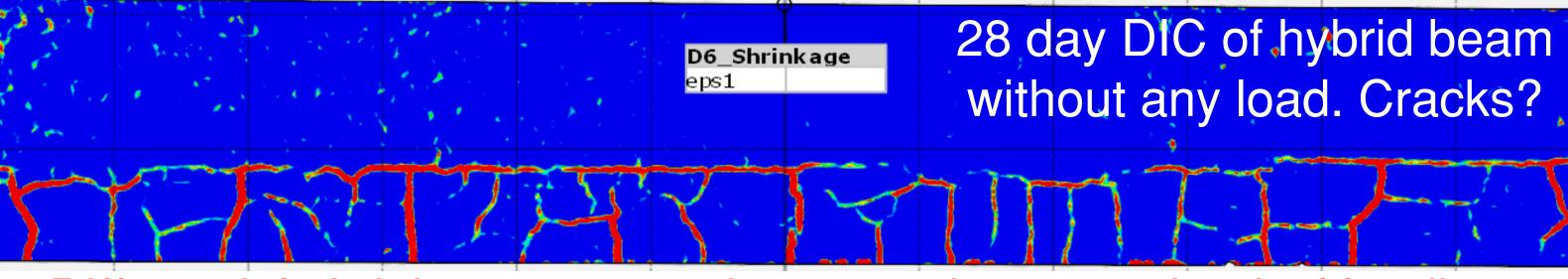
Differential shrinkage causes damage prior to mechanical loading.
