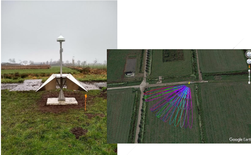
Figure 3 – Left: Picture of the ZGVLD GSNN antenna and two corner reflectors. Right: Reflection sensing zones, Zegveld.
