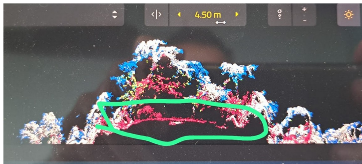
Terrace found in the UAV LiDAR data
