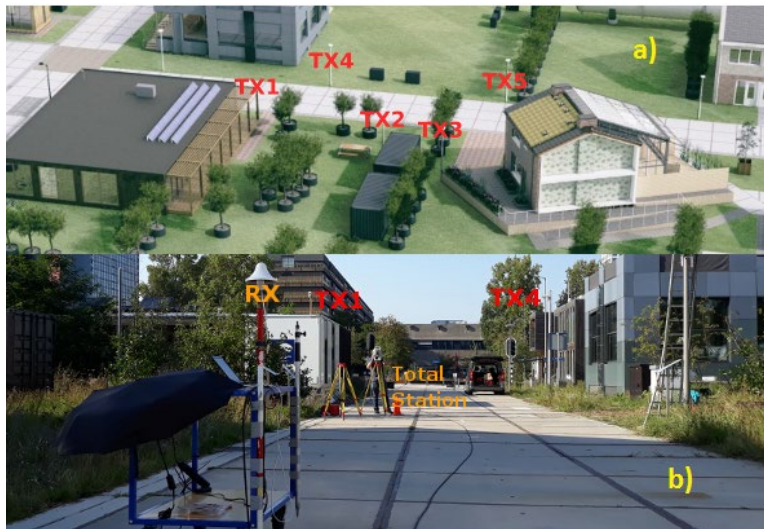
Figure 5: a) Geometry configuration of the five pseudolites, labelled in red. Four transmitting SDRs are used to serve 5 transmitting antennas, typically mounted in lampposts. TX2 and TX3 are both linked to a single SDR which is transmitting on its two channels. 1PPS and 10 MHz reference signals are provided by 4 timing nodes connected to the SDR systems. The receiver is moving on the road. The stretch of road covered by the transmitters is about 50 meters long, and 6 meters wide, b) Photo from the experimental test site, the transmitting antennas TX1 and TX4 can be seen. The receiving antenna mounted on a trolley, and the Total Station used to measure its 2D position is shown as well.
