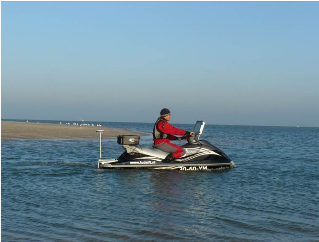
Fig. 16: A water scooter, equipped with an echo-sounder is used to monitor the sand engine (zandmotor), near the Dutch coast. High-precision GPS - note the antenna at the back of the water scooter - is used for positioning, in order to turn the echo-sounder depth-measurements into a sea-floor-map. Image courtesy of Matthieu de Schipper.
