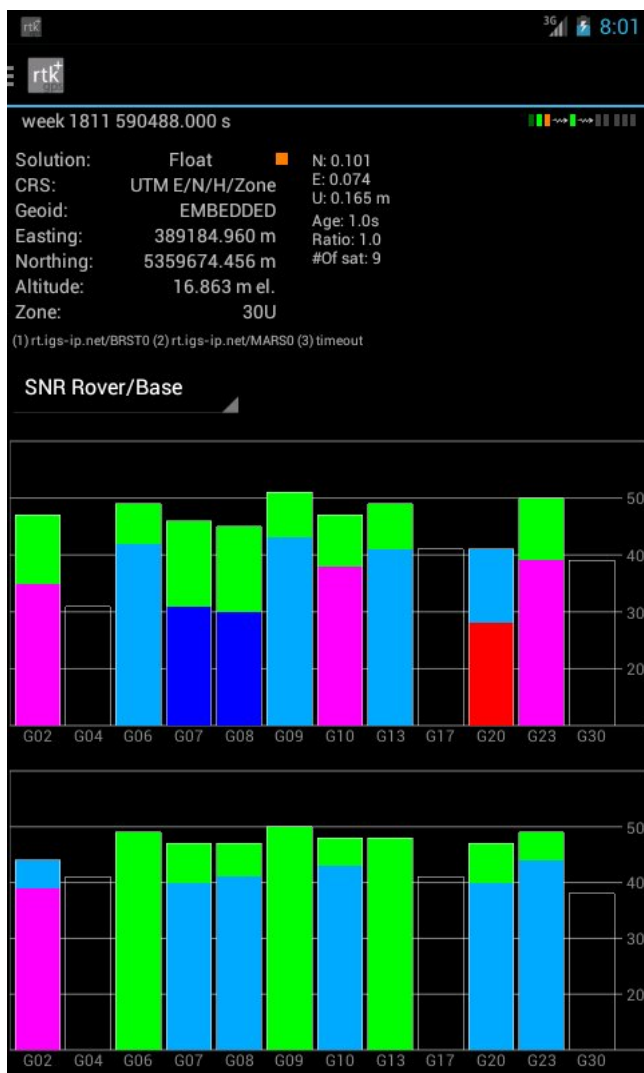
Fig. 12: RTKGPS+ , an Android port of the RTKLIB software, brings high-accuracy positioning techniques to the smart phone. Note: the software relies on an external GPS device to obtain the pseudorange and carrier phase measurements. Image source: appstore .
