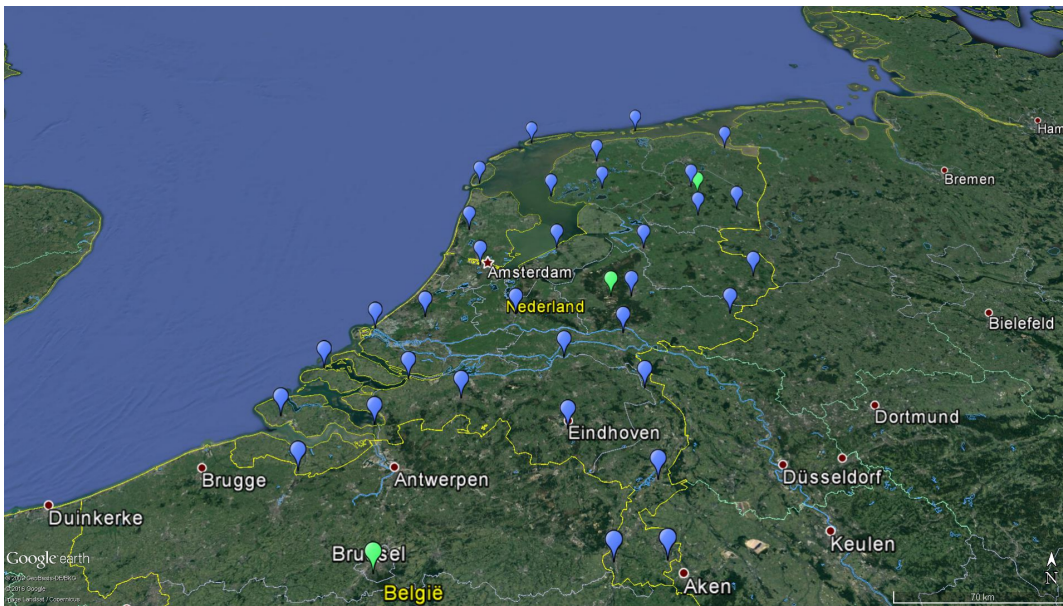
Fig. 10: Example of a dense local GPS reference network used for RTK in the Netherlands in blue, and a sparse global network used for PPP in green (figure created with Google Earth™).
