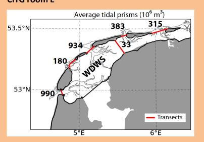
In barrier-island systems like the Dutch Wadden Sea, large amounts of water are exchanged through the inlets with every ebb and flood (this amount is called the *tidal prism*). But one may find that, on average, flood dominates in some inlets, while ebb dominates in others. In that case, there is a residual flow through the system, i.e. there is a net flow if one integrates over a tidal period.
