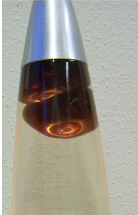
Figure 5. Two blobs prevented from merging by a thin film of water.
