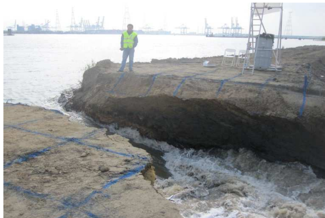
Figure 3: Full-scale breach experiment near Fort Lilo (Belgium) by Flanders Hydraulics Lab and TU Delft.
