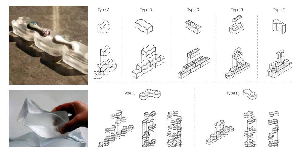
forms are kilncast in 1:2 scale. The components are then dry-assembled in series of three and structurally tested under shear, to demonstrate the
