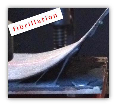
A generic adhesive zone constitutive model is introduced to describe the process of membrane debonding on the basis of fibrillation.
