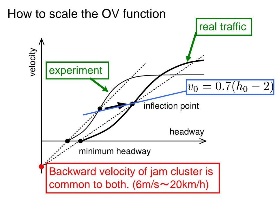
Relations between  $\alpha', \beta', h_0', v_0'$  and  $\alpha, \beta, h_0, v_0$ (real traffic) (experiment)  $V(h) = \alpha \tanh[\beta(h - h_0)] + v_0$  $\alpha' = \frac{v'_0}{v_0} \alpha$  $\beta' = \frac{h_0 - h_{\min}}{h'_0 - h'_{\min}} \beta$  $h_{\min}' = \frac{v_{\text{back}}}{v_0' + v_{\text{back}}} h_0'$  $v_0' = 0.7(h_0' - 2)$
