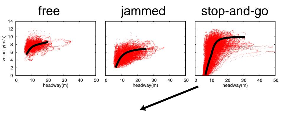
We can determine the OV function only in the case of stop-and-go flow.
