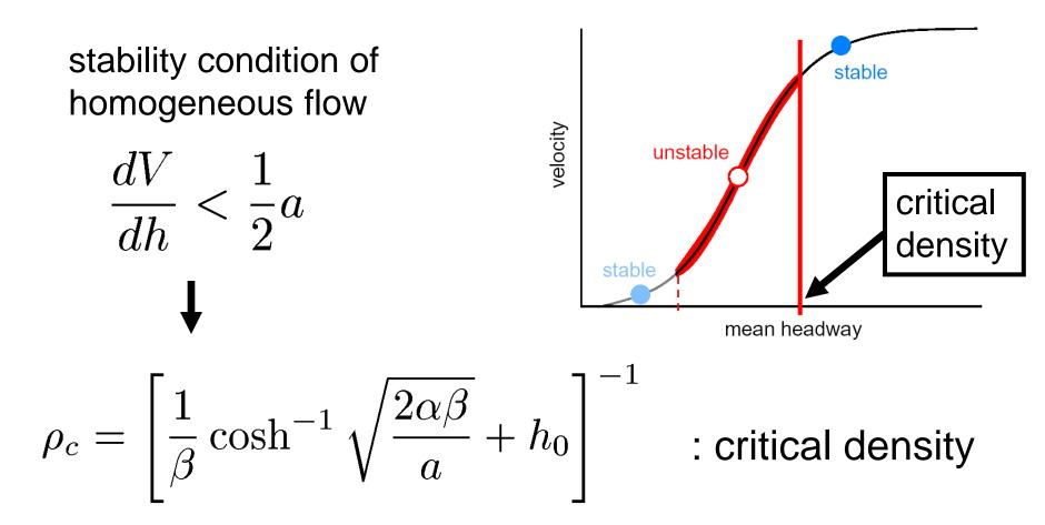
The difference in OV function explains the difference in critical density between experiments and real traffic.
