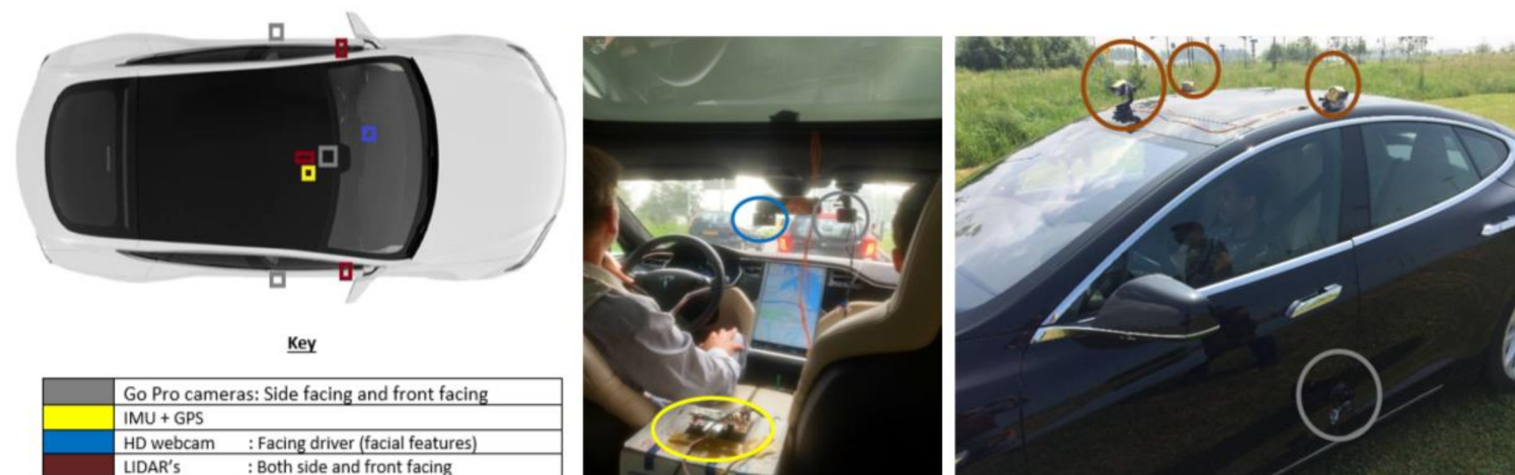
Figure 2: Illustration of vehicle instrumentation.
