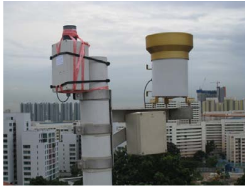
Figure 27: Disdrometer located next to tipping bucket, Singapore
