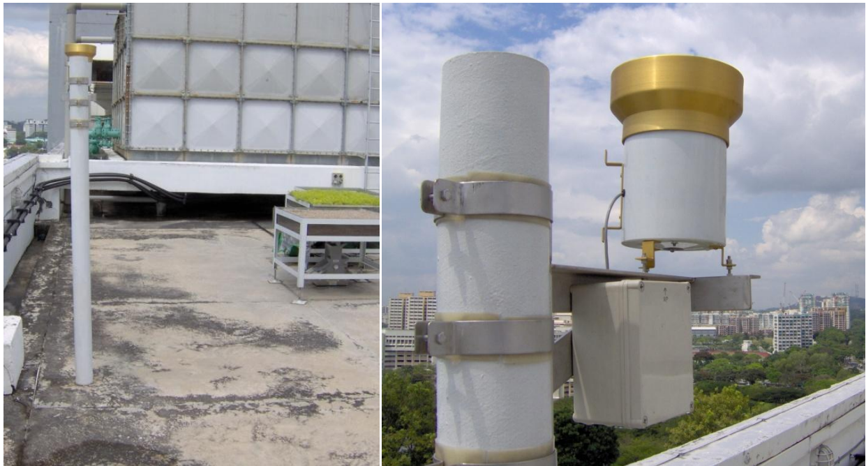
Rainfall is measured with a Global Water tipping bucket and data logger
