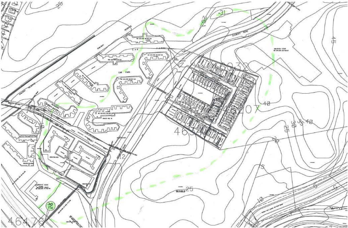
Map including contour lines, subcatchment demarcation (green dashed line) and outflow point at the main canal (left bottom)
