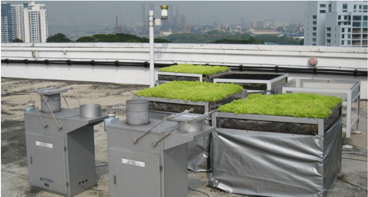
Figure 20. Green roof experiment set-up
