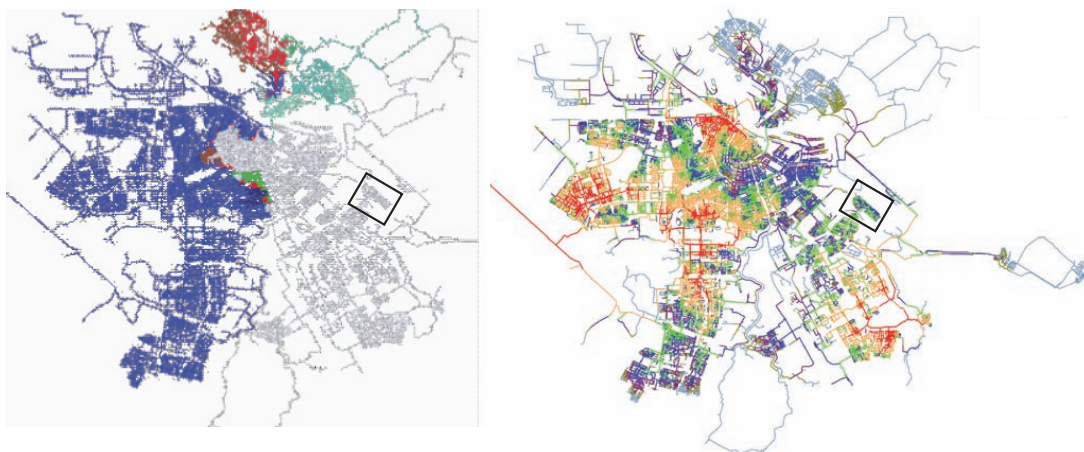
Figure 3.5: Mixing zones and average age of the water from Leiduin and Weesperkarspel. - The left picture shows the water origins. The probability that the water comes from Weesperkarspel: blue (less than 1%), green/red (40-50%), white (more than 90%). The right picture shows estimated average hydraulic residence time in Waternet network. The colours in the legend represent hours during which water remains in the pipes: minimum residence time, red (<5 hours), minimum residence time, grey (>30 hours and more). Source: Waternet.
