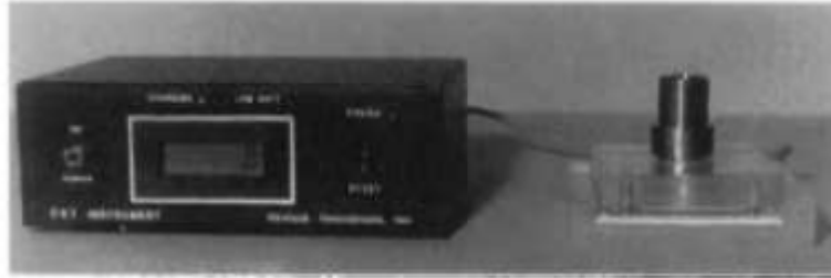
Figure 2-7 Capillary Suction Time Apparatus (to be replaced with original pic of device in lab)
