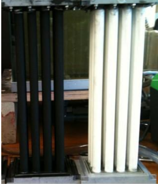
Figure 10: Blank membrane (right) and pre-coating membrane (left)
