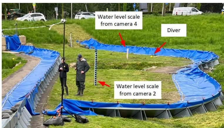
Figure 20: Location of the water level scales and the diver
