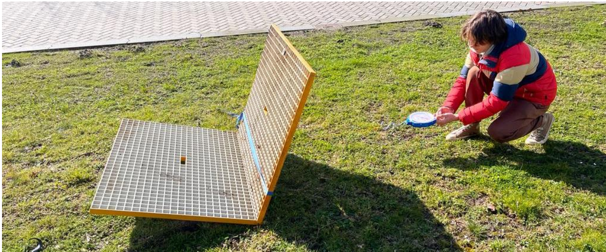
Figure 10: Tilting of test setup of friction measurement (Hemmes, 2023)
