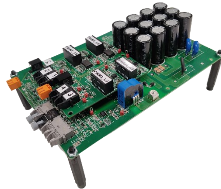
(b) Possible H-bridge Solution
