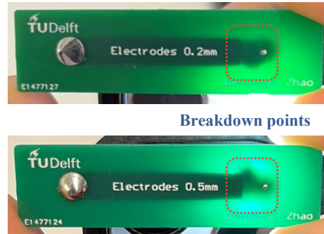
Fig.2 Breakdown of PCB electrodes (FR4)
