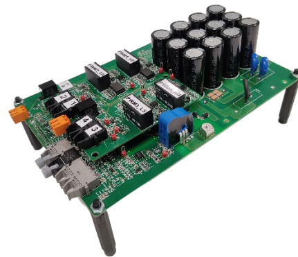
(b) Possible H-bridge Solution
