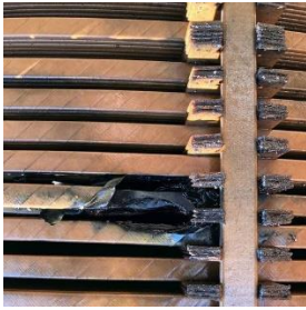
Figure 1. Inter-turn fault [electricaltechnology.org].
