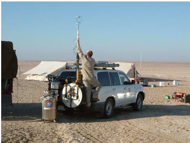
Figure 2. The laser diode spectrometer, control hardware, gas handling system, data logger and liquid nitrogen supply are mounted in an off-road vehicle. Although the instrument is operated continuously, best noise performance is obtained with the vehicle stationary. Typically 15 minutes of data are recorded at each measurement position. A telescopic mast places the sample inlet and anemometer 5m above the ground.
