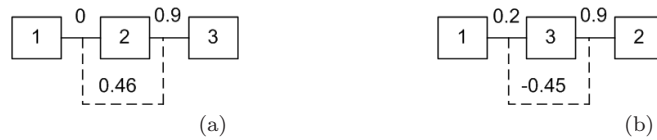
Fig. 1.2. D-vines "representing" induced and non-transitive dependencies. (a) D-vine representing the independence of X_1 and X_2 . (b) D-vine representing the conditional dependence of X_1 and X_2 given X_3 .
