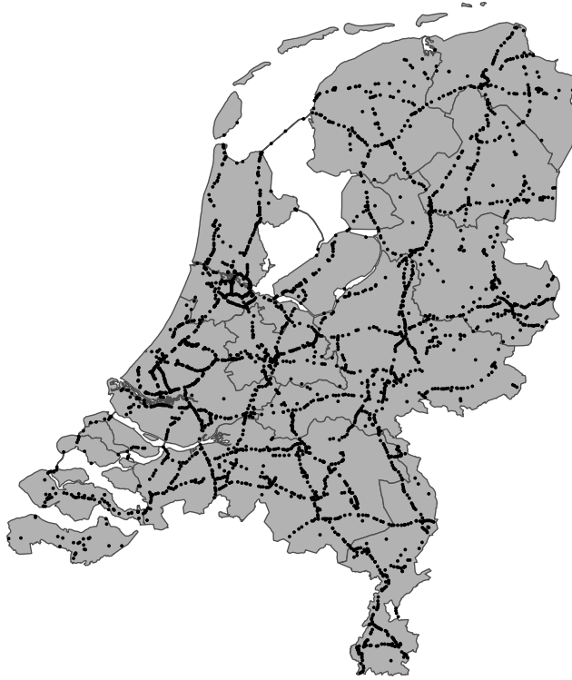
FIGURE 1.3: Map of the Netherlands with the location of bridges which are managed by the Civil Engineering Division.
