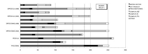
FIGURE 2. Experiment 1: Wall clock time for different stages of PCG and DPCG for  $TOL=10^{-2}$ ,  $10^{-6}$ .
