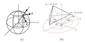
FIGURE 9. (a) spherical coordinates, (b) rotation around origin of tetrahedral element in x, y-plane
