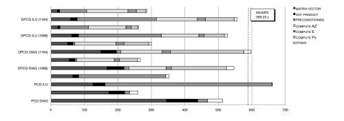
FIGURE 5. Experiment 2: Wall time for different stages of PCG and DPCG for  $TOL=10^{-2}$ ,  $10^{-6}$
