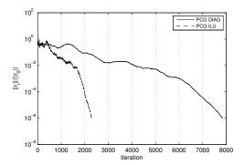
FIGURE 3. Experiment 1: convergence curve of the PCG method for diagonal scaling and Incomplete Cholesky preconditioners
