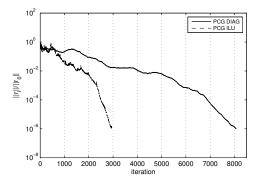
FIGURE 7. Experiment 2: convergence curve of the PCG method for diagonal scaling and Incomplete Cholesky preconditioners
