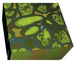
FIGURE 1. FE mesh that consists of 7,977,448 elements representing cube of asphaltic material containing aggregates (light green), bitumen (dark green) and air voids (blue).
