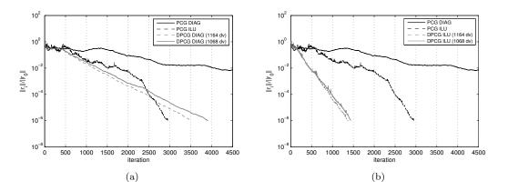
FIGURE 8. Experiment 2: convergence curve of the DPCG method for diagonal scaling (a) and Incomplete Cholesky (b) preconditioners compared to the PCG method (diagonal scaling and IC)
