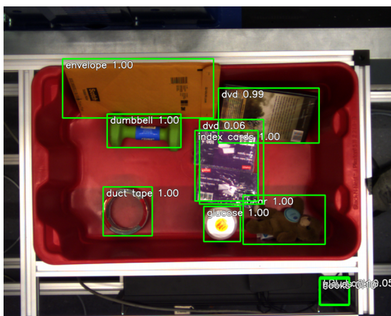
Pictures of the deep learning object classification (left) and robot system (right) with which we won the Amazon Picking Challenge 2016.
