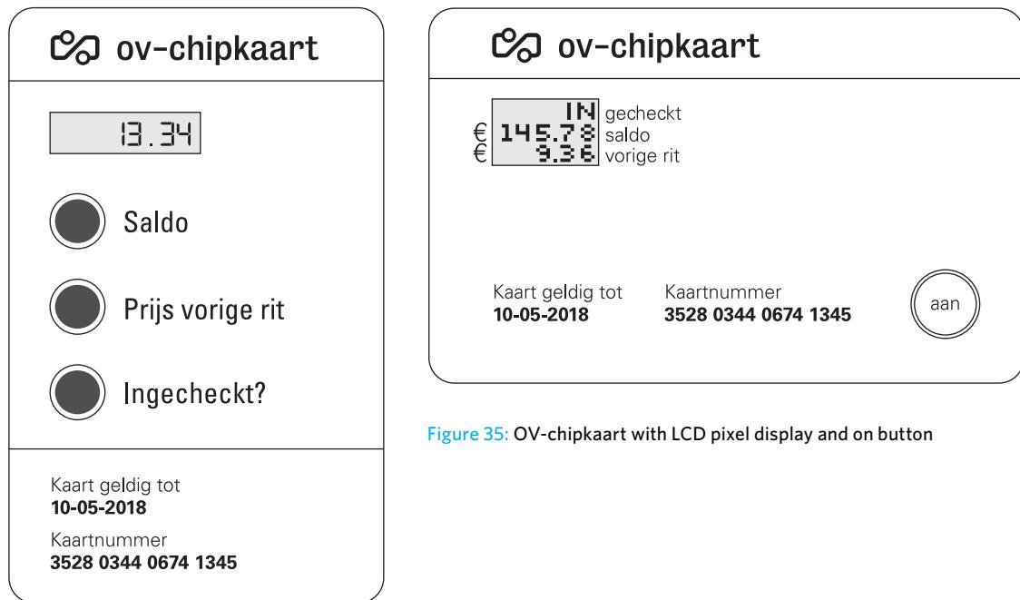
Figure 34: OV-chipkaart with LCD segmented display and single function buttons
