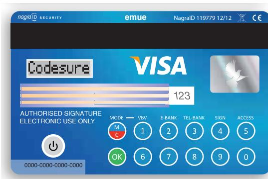
Figure 21: Nagra ID Codesure creditcard with LCD pixel display and keypad
