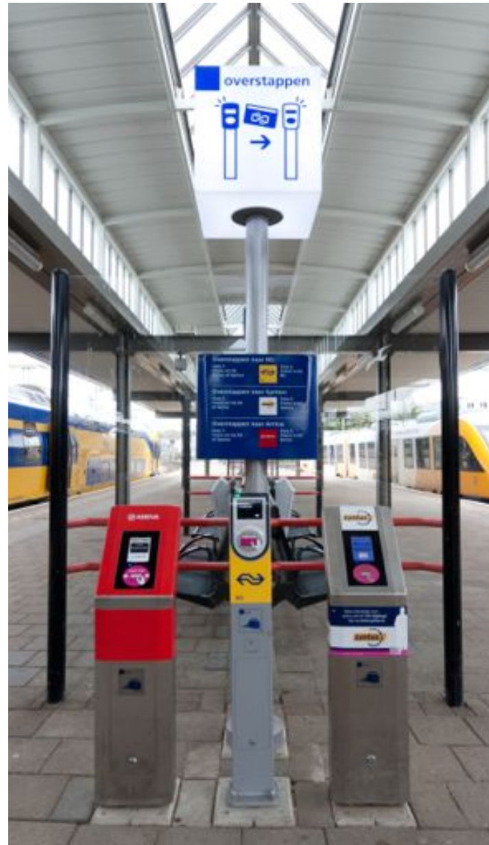
Figure 14: Validators from three different train operators at a train station. This is an invisible payment border.
