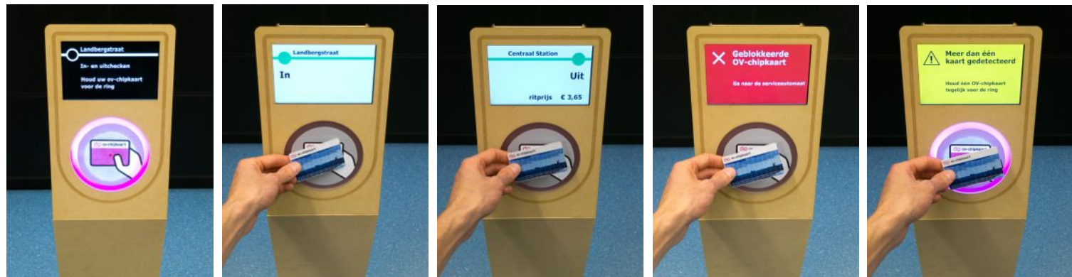
Figure 45: Top part of the prototype. The LED ring switches on when a smart card is read. The LED ring flashes when the user needs to perform an extra or repeated action.
