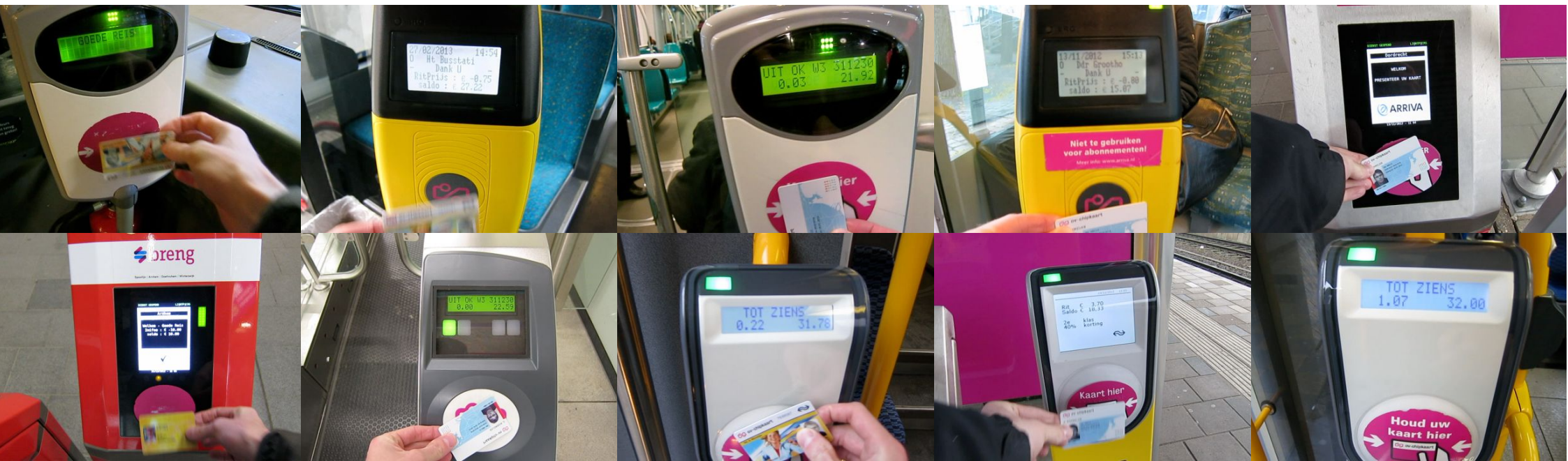
Figure 28: Screenshots of movie clips of check-in and check-out actions: a variety of display types and feedback signals.
