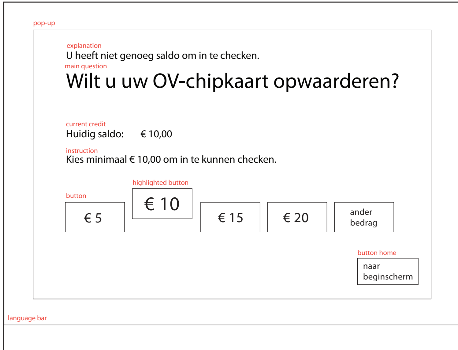
Figure 39: Wireframe of a service machine screen. This is the first screen when tapping the OV-chipkaart at the ticket machine after an 'too little credit' error at a validator.
