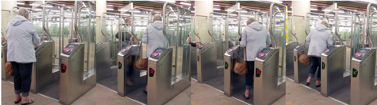
Figure 27: A traveller checked in at the wrong gate, she did not understand which RFID reader belonged to the gate.
