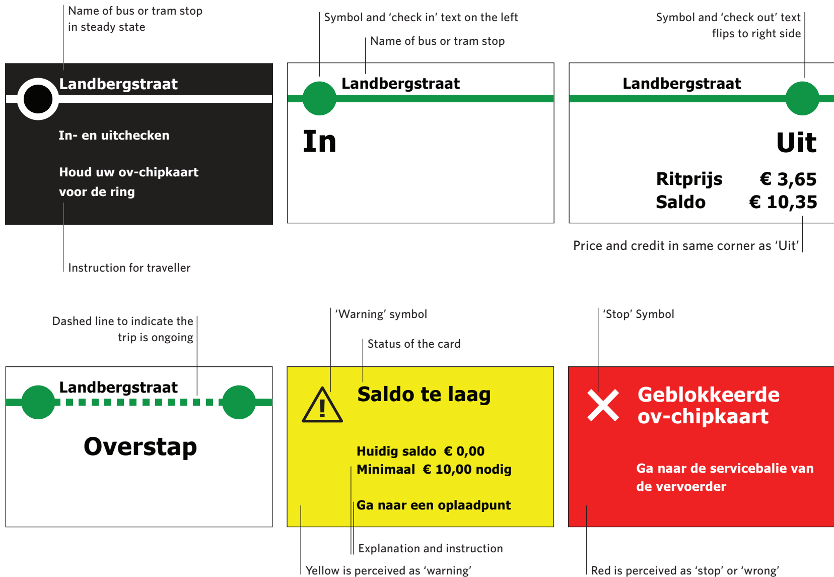
Figure 35: Six different messages to display: 'standby', 'check-in', 'check-out', 'transfer', 'error but can be solved quickly', 'severe error'.
