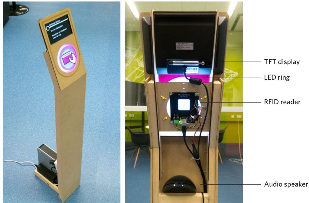
Figure 44: Interactive prototype of a validator, left: the front side, right: the back side showing the different components.
