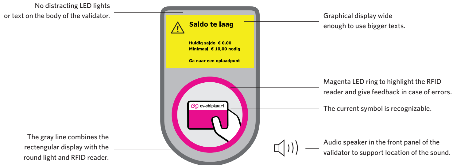
Figure 36: Input and output components of a validator. This is comparable to Thales V4 equipment, but with some changes: LED ring added and extra light signals removed.
