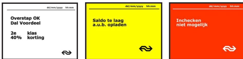
Figure 9. Examples of messages the display on the gate can communicate: validation successful (white), validation unsuccessful (red) and another step is needed (yellow)
