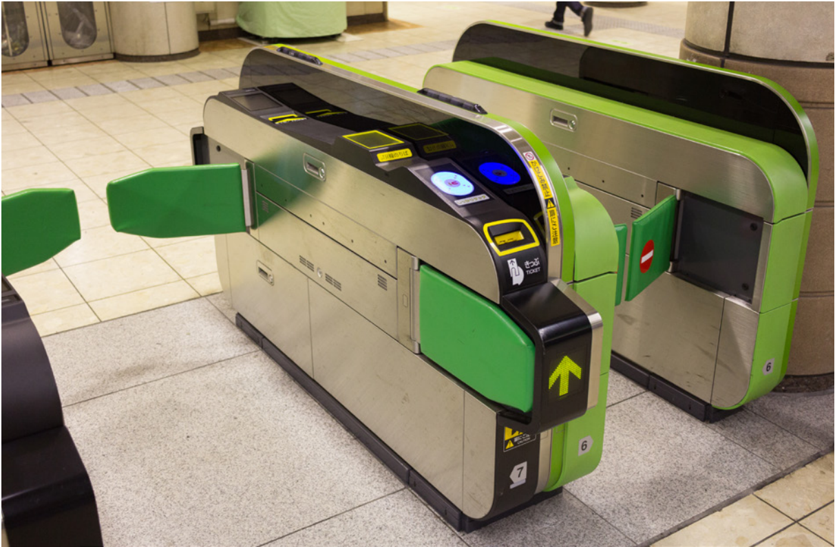
Figure 48. A gate of train operator JR in Tokyo. Notice the usage of colour, the doors on both sides of the gates, and the several elements on top of the gate
