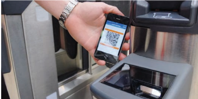
Figure 3, Gate with scanner
