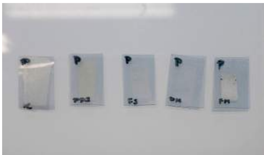
Fig146Preparing the samples. Keeping track of the PET side by writing a P on that side. When placed on top of each other both P's should align indicating both an ITO and PET side are facing the HMA.
