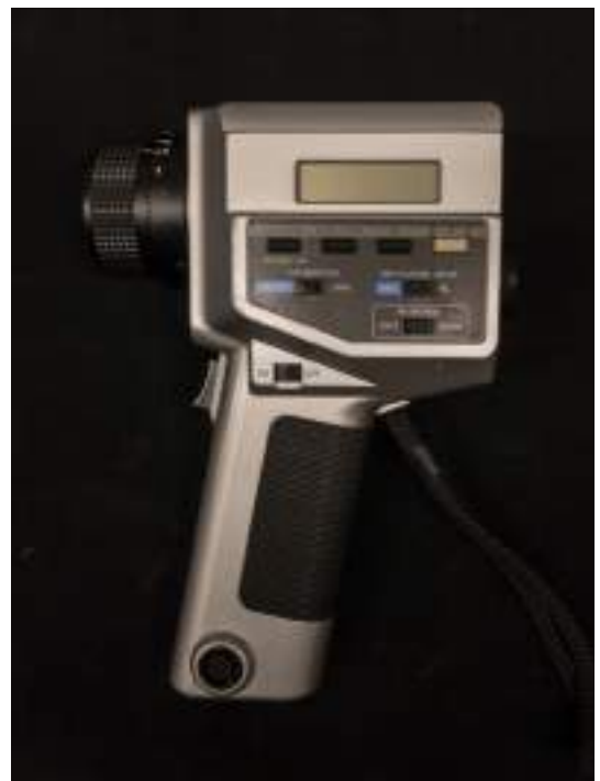
Fig165Minolta luminance meter LS-100.
