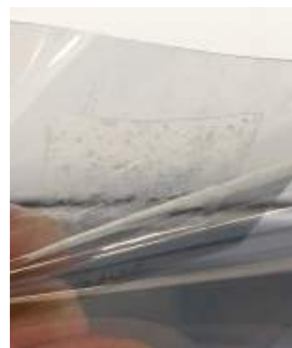
Fig147Delamination of Digimount, showing poor adhesion to ITO.
