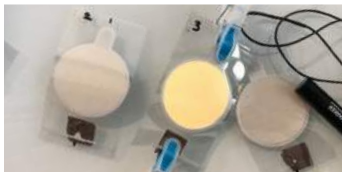
Fig18. The test resulted in only one working device. This is the one with three dielectric layers applied. The others did not emit light at all.
