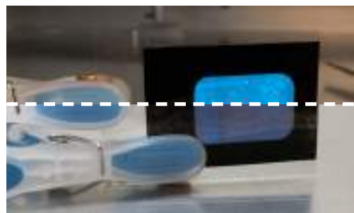
Fig94. Copper as electrode yield a low emission compared to aluminium. The top half is perception in a dark room, the bottom in a room with the light turned on.
