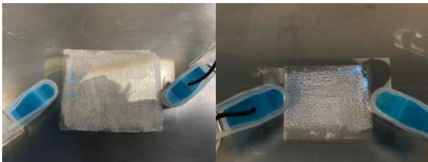
Fig152Right: Second method for using HMA to trap phosphor particles, distance between the electrodes at the brightest emission center is 55 micron.
