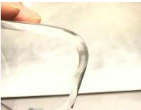
◀ Fig77. Delamination after only a small amount of force is applied.
