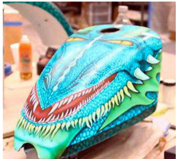
Fig22. Covering a motorcycle tank with EL spray paint for 3d-curved surfaces.
