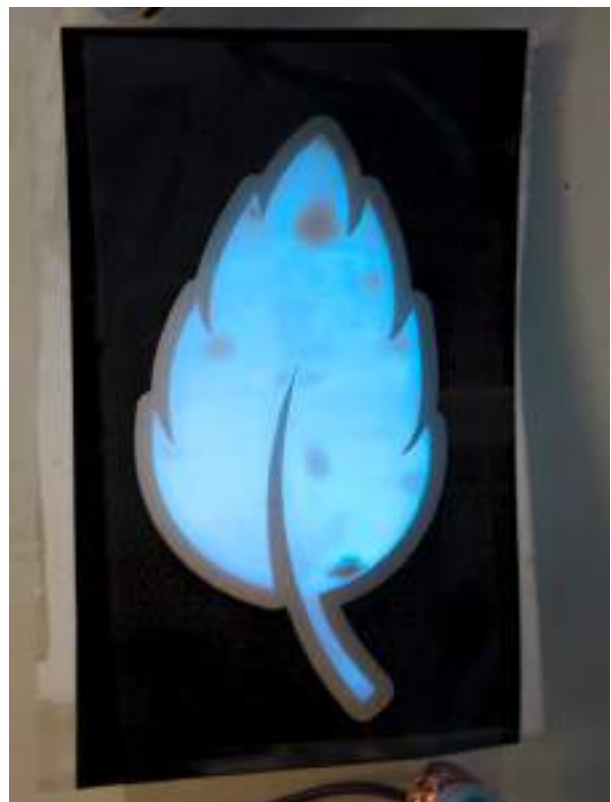
▼ Fig137. Results using the UV method. Dark spots are caused by small particles on the working area.
