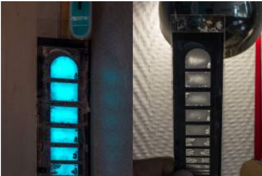
Fig160Bison sample turned on and held against the light. It is clearly visible that the brighter parts are more transparent. Measurements showed that these parts are also significantly thinner.
