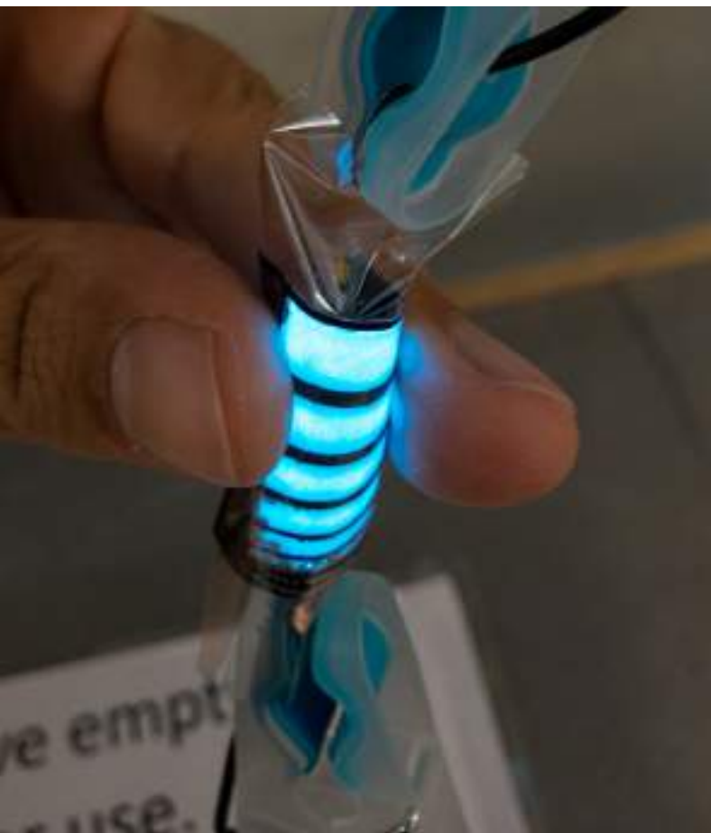
Fig80. Properties of this construction are, high output, very flexible and no need for a separate dielectric layer. The 25 micron ITO PET (left) is significantly more flexible than the 125 micron ITO PET (right)
