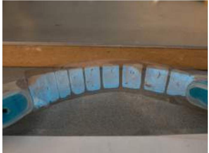
▲ Fig81. Loss of output and details if the PET is used as dielectric.
