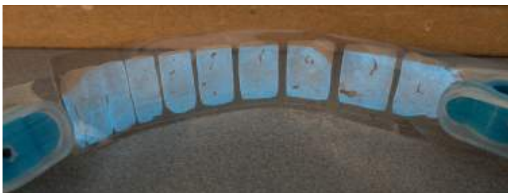
Fig163 The top part of the sample does not emit light because the top piece of ITO PET was cut to narrow. The top part is above the red line.
