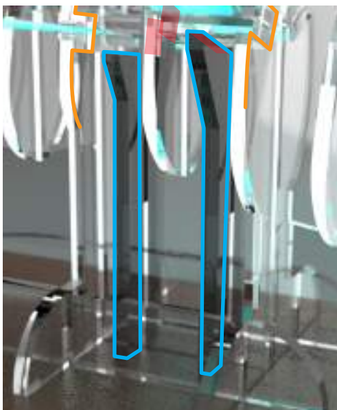
▼ Fig148. Supporting structures underneath the wings (made black to make them stand out more).
