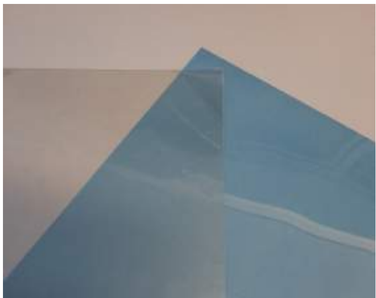
▼ Fig32. A sheet of ITO PET. This supplier has covered the conductive ITO side with a blue protective foil which has two functions, protection the ITO layer and it works as an indication of which side is the ITO side. It is not possible to determine which side is the ITO side by sight. Some supplier cover both sides with a similar coloured foil which means the conductive side needs to be determined manually. This can be done by attaching two pieces of conductive copper tape and use a multi meter to measure the resistance.
