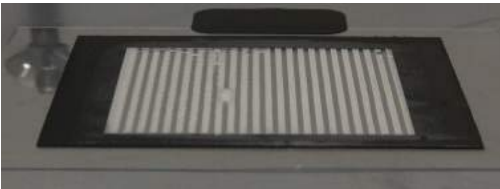
▼ Fig112. Shot at a steep angle this image clearly shows much cleaner lines in the right half of the sample.
