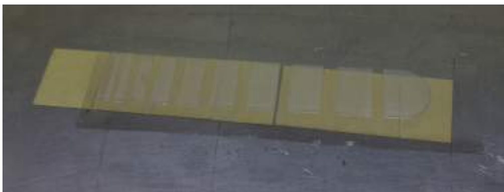
Fig162 Removing the vinyl left the deposited untouched. Providing clean straight lines.
