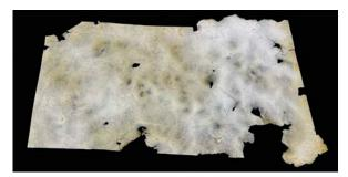
Bio Mineralized Bacterial Cellulose Material
