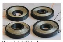
3D printed coils for Wireless Power Transmission system
