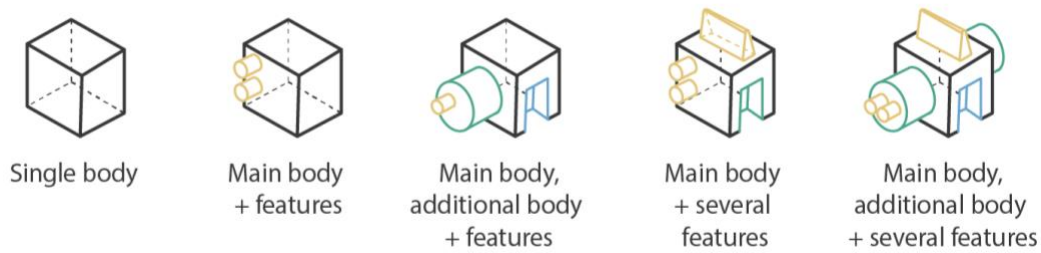
Figure 6 - Part complexity type, based on Repair Using 3D printing by Thijs Beerkens [1] .
