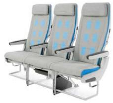
Flightbeat is a platform that monitors the wellbeing (physically and mentally) of passengers through heart rate sensors, which are integrated
