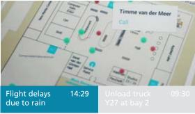
Envisioning a cargo warehouse of the near future, we developed an autonomous pallet transport system for KLM Cargo. With the use of Google Glass and Android tablets, workers can control a network of robotic vehicles, from a shared working environment. With everything and everyone connected in real-time, productivity is improved.
