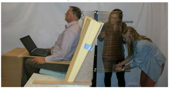
In this research, the head, neck and back contour of a human while sitting in two different aircraft seats, performing two tasks (namely watching in-flight entertainment (IFE) and working on a laptop) are estimated by using a kyphometer. The research question was to find if anthropometric properties, the design of the chair and the performed activity has influence on the back contour of a person. This research
