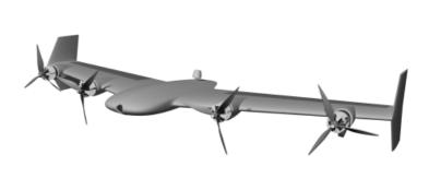
The Peregrine drone consists of a 69 cm swept wing, with a main pod to accommodate for storage of the electronics and battery at a suitable center of gravity. Double-sided winglets are present to allow for stable landing and takeoff in a tail-sitting configuration. To fulfill the mass budget, the structure of the drone is a composition of carbon-fiber
