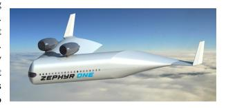
Using Differential Evolution with custom built-in design iteration, the aircraft design is optimized to have minimal fuel burn over its entire mission. This approach optimizes the engines, the wing planform as well as the cruise altitude and velocity for minimum fuel burn, yielding incredible performance that could never be achieved by manual design-iterations.
