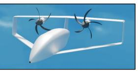
equal to 1,193 kg, of which 115 kg are due to the fuel cell, 30 kg of hydrogen mass and 53.5 kg of batteries. The Prandtl plane has a cruise altitude of 12.5 km, a cruise speed of 163 m/s and can complete the race without any stops in 216 minutes (slightly over 3.5 hours).
